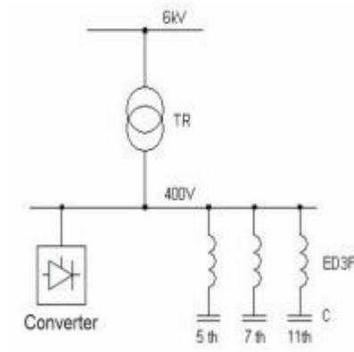
*Drawing 1 Simplified diagram for the reactive power compensation circuit and harmonics filtration [on the basis of literature].*
