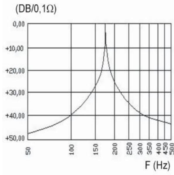
*Drawing 3. Suppression characteristics for LC system with a protective choke with the ratio  $p=7\%$ . [on the basis of literature].*
