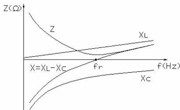
*Drawing 2. LC filter impedance characteristics [1].*
