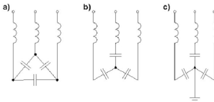
*Drawing 4. Selected LC passive filters systems [on the basis of literature]*
