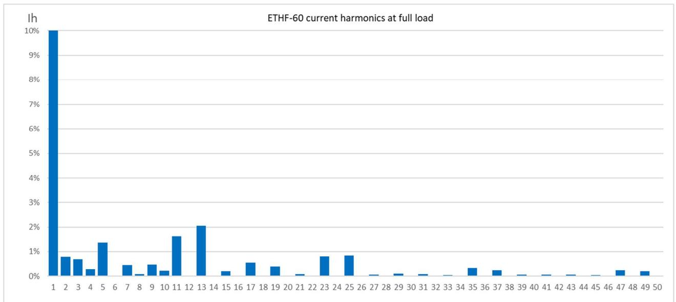
Figure 7: Harmonics Spectrum up to 50 at full load
